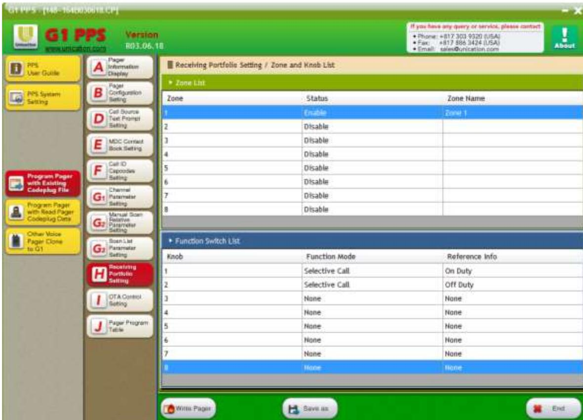
With this configuration when Selector Switch knob is set to position 1 any received message will alert (because the Call ID on this channel did not have the “Off Duty” clicked). In knob position 2, the Call ID on this channel has “Off Duty” selected and since in Step 1 the Default Setting for the G1 was set to “Off State” any messages will be received and stored **without** an alert.
